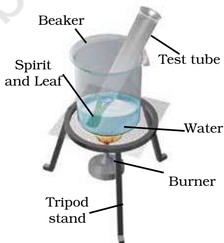
Figure 4.1 Set-up for extraction of chlorophyll
