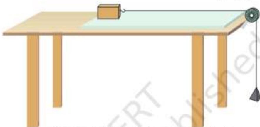
Fig. 35.1 : Experimental set up to study variation in limiting friction with the mass of the object suspended
