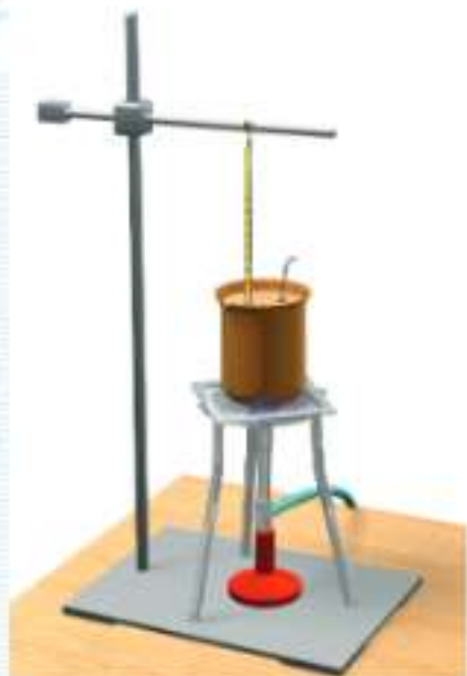
Fig. 38.1 : Heating of water in a calorimeter.
