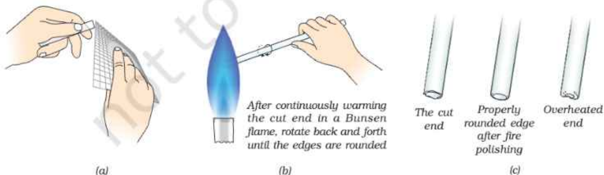
Fig. 2.2 : (a) Trimming the jagged edges (b) Rounding the edges (c) Properly and improperly rounded edges
