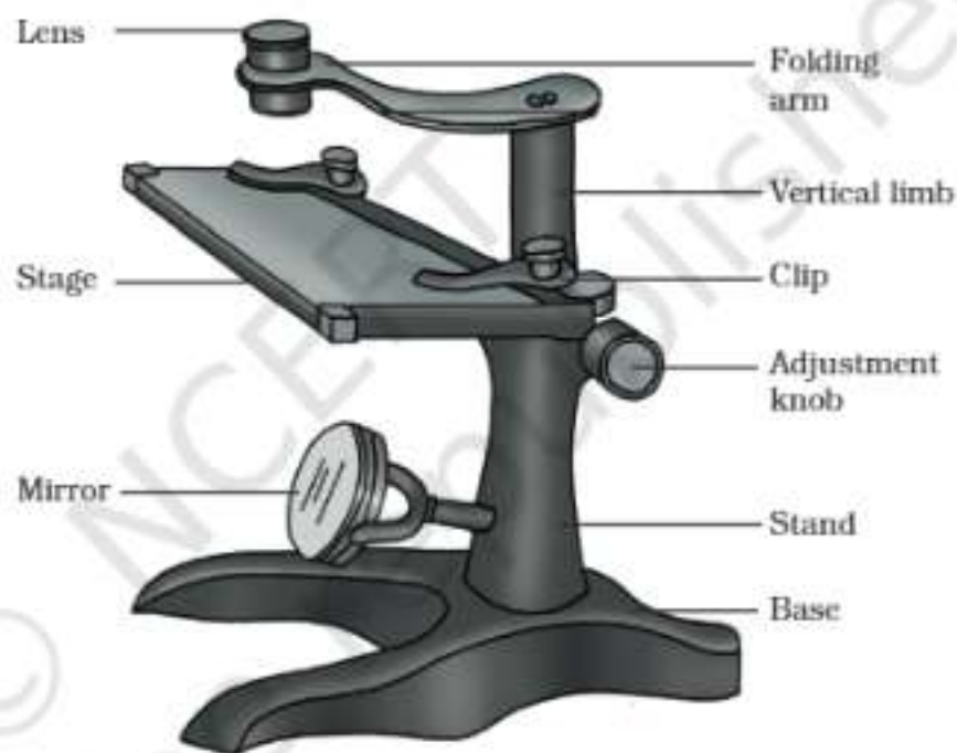
Fig. 1.1 : A simple (dissecting) microscope
