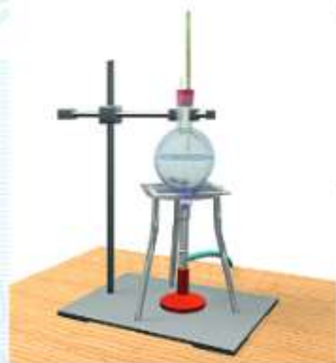
Fig. 8.1 : Determination of Boiling point of water
