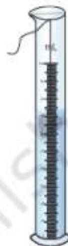
Fig. 4.2 : Determination of volume of a non-porous solid
