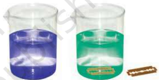
Figure 18.1 Change in colour of the copper sulphate solution due to reaction with iron (shaving blade)
